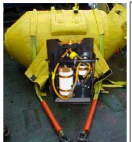
The Ordnance Automatic Recovery System (OARS) is a "lift and descend" self inflating air bag system allowing for the controlled subsea and surface movement of UXO Ordnance.
