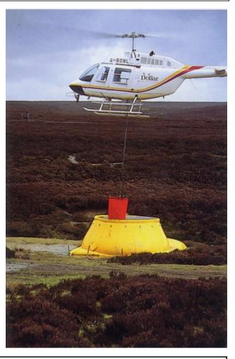
Flexi-Dams are self supporting liquid containers with an inflatable collar, ready for instant deployment to safely hold water, chemicals, fuels, pollutants and more. Used in a wide range of environments, they are popular with Emergency Services globally due to their light weight and compact stowage, making them an essential part of the fast response to situations.
